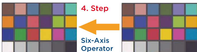
Figure 9: Illustration of the four steps towards a good color calibration: White balancing, gamma correction, matrix correction and correction by the six-axis operator
