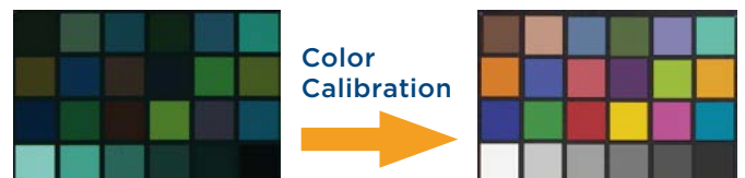
Figure 8: Greta Macbeth ColorChecker®, recorded with the uncalibrated camera (top) and shown with the theoretical target values (bottom)
